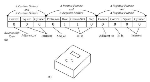
Fig. 4. (a) Binary code-based representation of functional features for the part shown below and (b) sample part.
