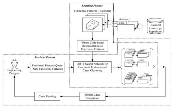
Fig. 2. Functional feature-based reference design retrieval process.
